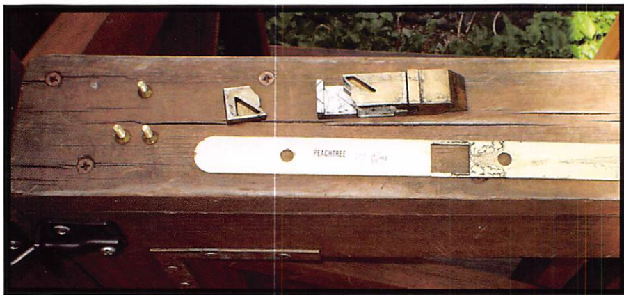
The mortise faceplate and the broken parts from the upper control module.
